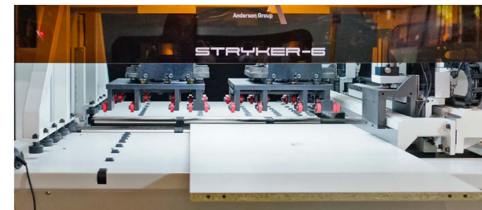
In-Feed system with rubber roller on working table
