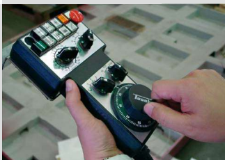
Hand-held device for easier machine operation
