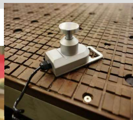
Touch-off device for Tool length measurement
