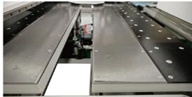
**Air-floating table design**, to reduces friction and avoid the scratch on the surface of material.
