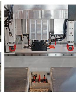
With 2 drill unit (from top and bottom), able to process 6 side of material in one pass, much improve the production efficiency.
