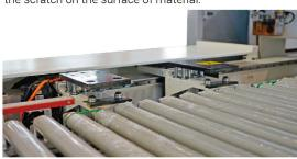
**Servo gripper feature,** machine is able to record the position of grippers, no need reference back and forth during working and no down time necessary.
